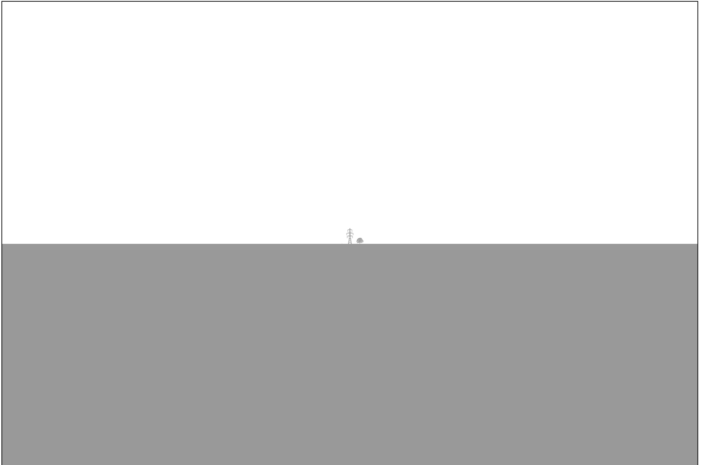
Pylon as appreciated when viewed at 3km distance (50m high pylon, 20m high tree, 1.8m high person)
